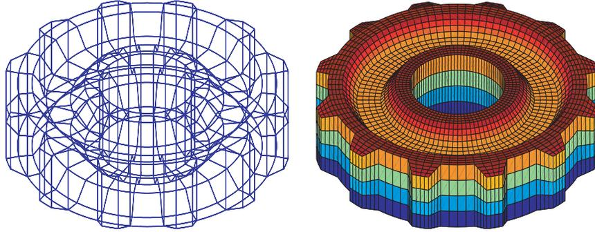
FIG. 1.1. A gearwheel represented by 336 patches and the associated mesh on the level 2.
