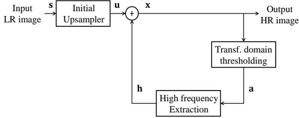
**Fig. 1:** Framework for image interpolation. A linear model, e.g., FIR filter is used to produce an initial upsampled image. Then, high frequency components are extracted after a sparsity promoting step and used to refine the initial upsampled image.
