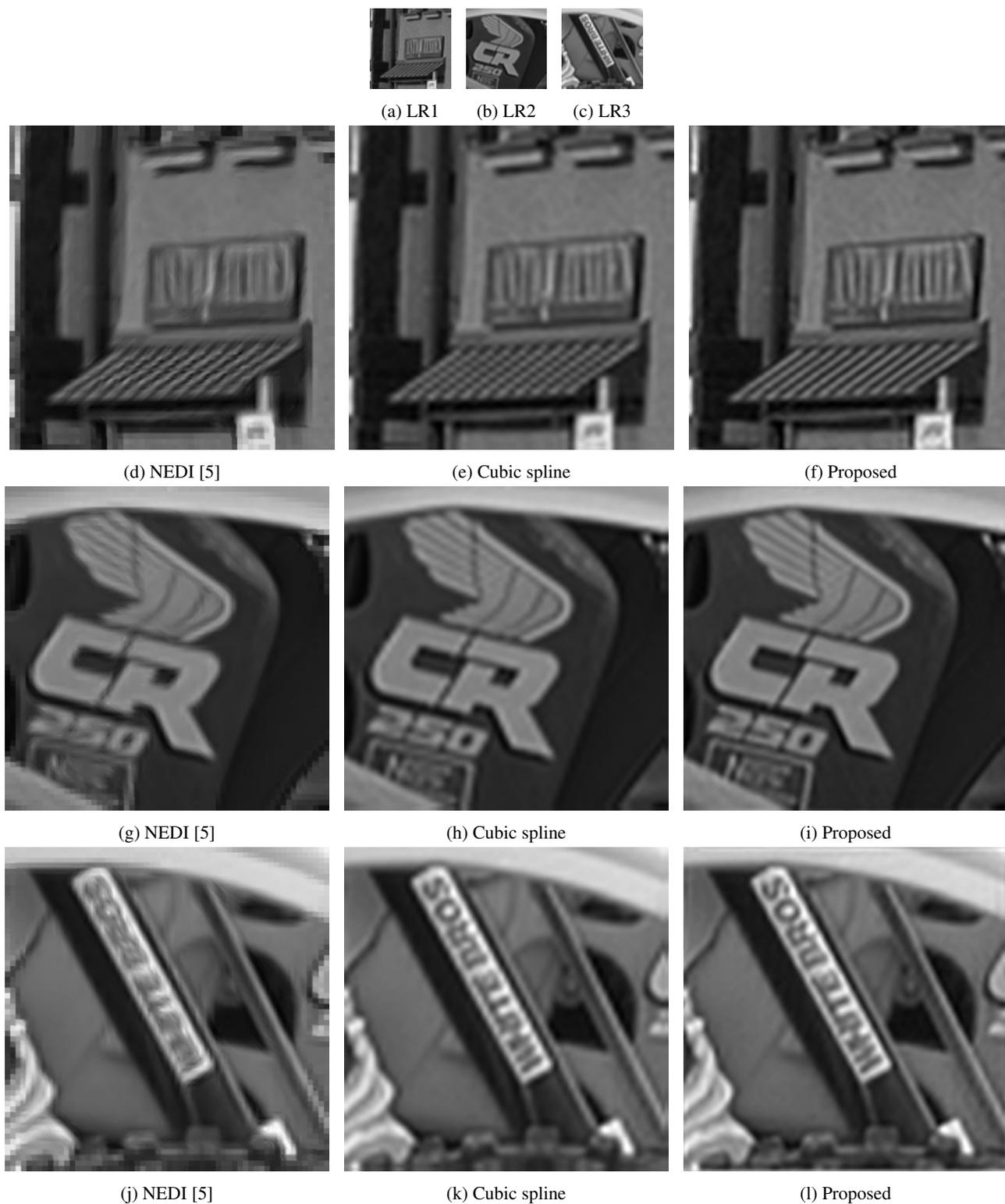
**Fig. 3:** Example 4x upsampling results (via successive application of 2x upsampling). Input patches of size  $64 \times 64$  are upsampled to  $256 \times 256$ . Left column results show jaggedness and other artifacts. Center column results are blurred. Right column results (proposed approach) appear slightly sharper without evident artifacts.
