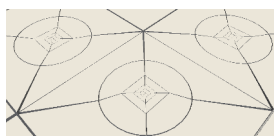
hp-adaptive FEM mesh for H_2O
